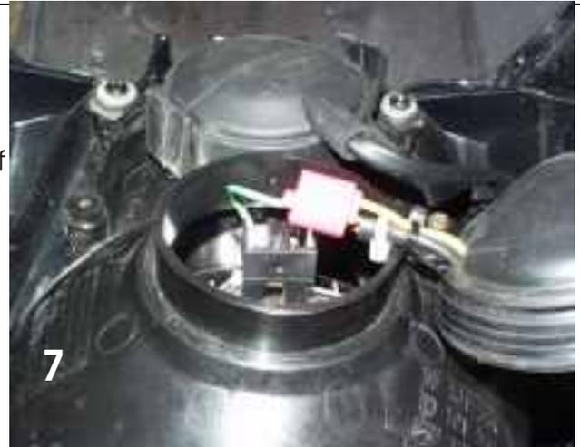
Shorten the blue and red cables as necessary (connecting fog headlights) and pull them through the slots provided on the underside of the fog lamp's back cover. Now attach the supplied flat connectors to the cables. Now attach the blue cable in the headlight to the outside right connector (ground).
