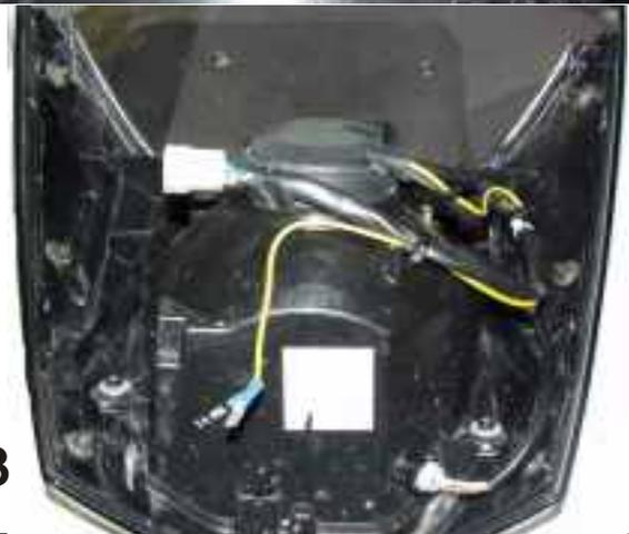
Attach the red cable directly to the bulb. Use a cable tie to secure the red cable to the light terminals. Now pull the cover over the headlight. Run the yellow cable to the dipped beam headlamp and connect it directly to the green cable located behind the lamp's connector using cable ties.
