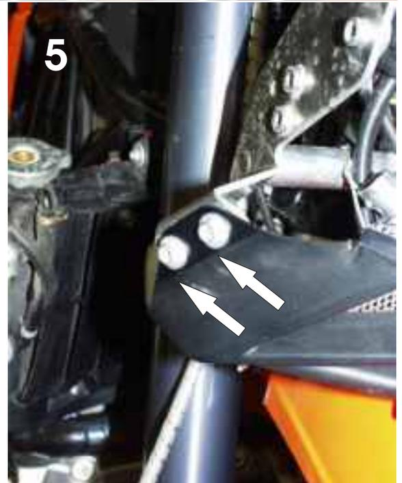
Bolt the U-shaped brackets to the headlights in such a way that the air exhausts are pointing downwards. Now bolt the U-shaped brackets of the headlights to the extra bulb fixture bracket and fit the fog headlight.
