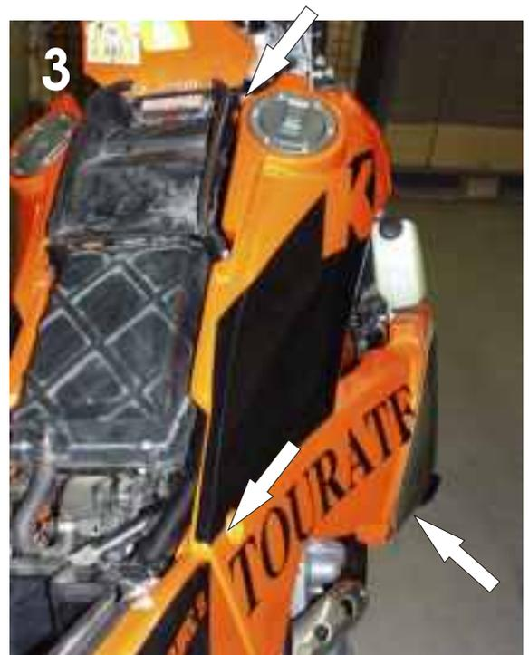
Close both fuel valves on both tanks and loosen the the screw connections on the right hand tank. Remove the right-hand tank and detach the hoses.
