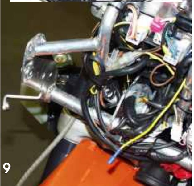
To make headlight assembly easier, you can shorten the yellow cable to the original height of the connector plug to the wiring harness and use a plug-in connection. Replace the original headlight on the fairing support, connect up the battery and test and adjust headlights.
